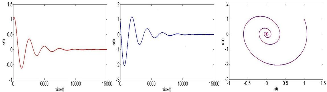
Figure 5. Under Damping
