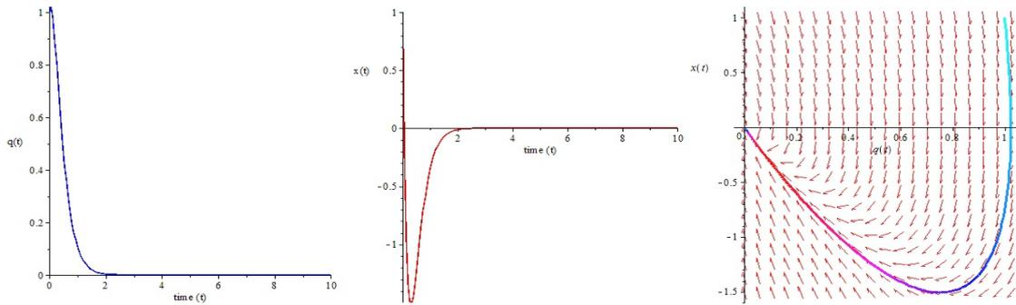
**Figure 4. Critical Damping**
