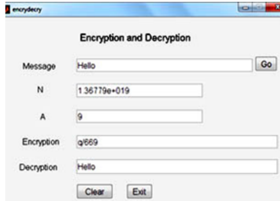
Figure 2. Encryption and decryption process of input message in MATLAB.
