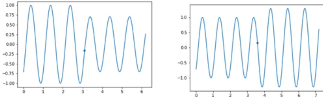
**Figure 3.** Illustration of the dynamics of the platform when subject to an impulse at the time of the solid dot
