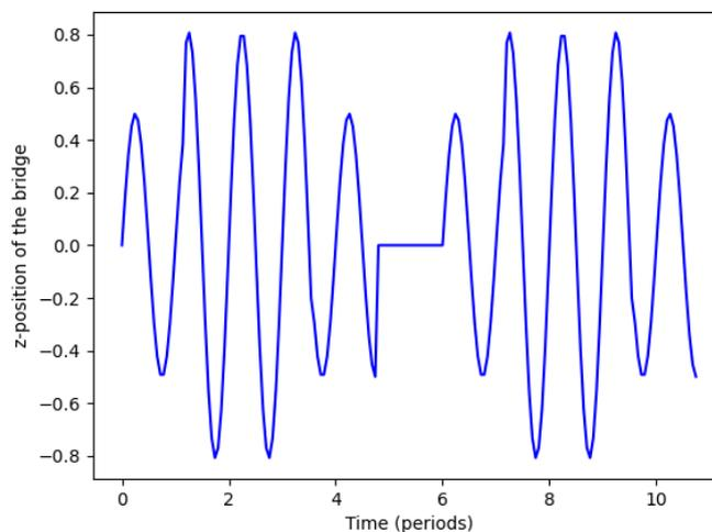
**Figure 4.** A plot of the  $z$ -position of the bridge under non-resonant conditions when  $\omega = 2\pi$  and  $T = 1.2$
