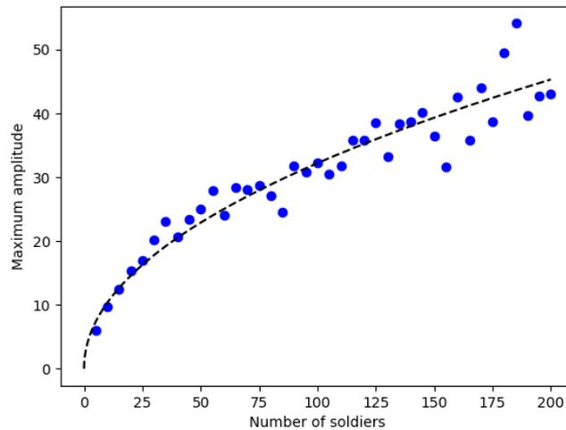
**Figure 5.** A plot of the maximum amplitude data when soldiers march randomly (blue dots) and the curve of best fit (black dashed line)
