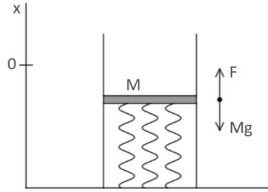
**Figure 1.** A spring model (simple harmonic oscillator) of the bridge
