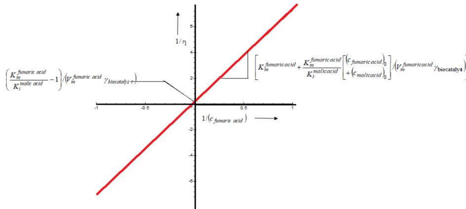
Figure 2: Estimation of kinetic parameters  $K_m^{fumaric\ acid}$  and  $K_i^{malic\ acid}$  using equation (19). The numerical value of the kinetic parameters used for the above figure is given in Appendix D.
