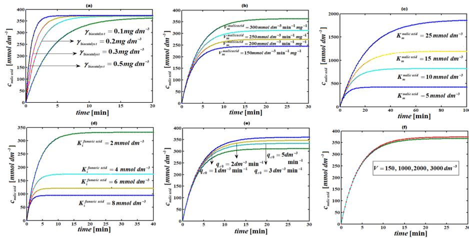
Figure 6: Concentration of malic acid in batch reactor versus time  $t$  for various values of parameter. Comparison between analytical result (Equation (12)) and simulation results. The numerical value of the kinetic parameters used for the above figure is given in Appendix D.
