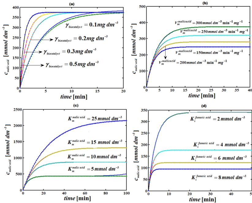
Figure 4: Concentration of malic acid in batch reactor versus time  $t$  for various values of parameters. Comparison between analytical result (Equation (10)) and simulation results. The numerical value of the kinetic parameters used for the above figure is given in Appendix D.
