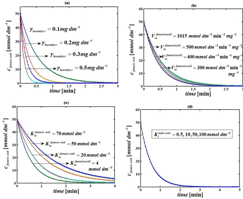
Figure 3: Concentration of fumaric acid in batch reactor versus time  $t$  for various values of parameters. Comparison between analytical result (Equation (9)) and simulation results. The numerical value of the kinetic parameters used for the above figure is given in Appendix D.
