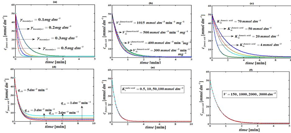
Figure 5: Concentration of fumaric acid in fed-batch reactor versus time  $t$  for various values of parameters. Comparison between analytical result (Equation (11)) and simulation results. The numerical value of the kinetic parameters used for the above figure is given in Appendix D.
