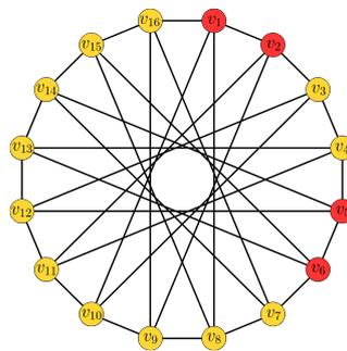
Figure 5: Perfect 2-coloring of  $Ci_{16}(1,7)$  with parameter matrix  $M_3$
